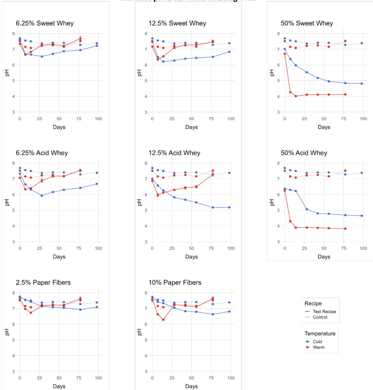
**Figure S1:** The pH of manure/additive mixtures over the course of the bio-acidification experiment. Additive percentages represent the amount of additive as a proportion of urine mass (50% indicates an urine:additive ratio of 2:1). Points each represent the average of three replicate tubes, and bars represent standard error.
