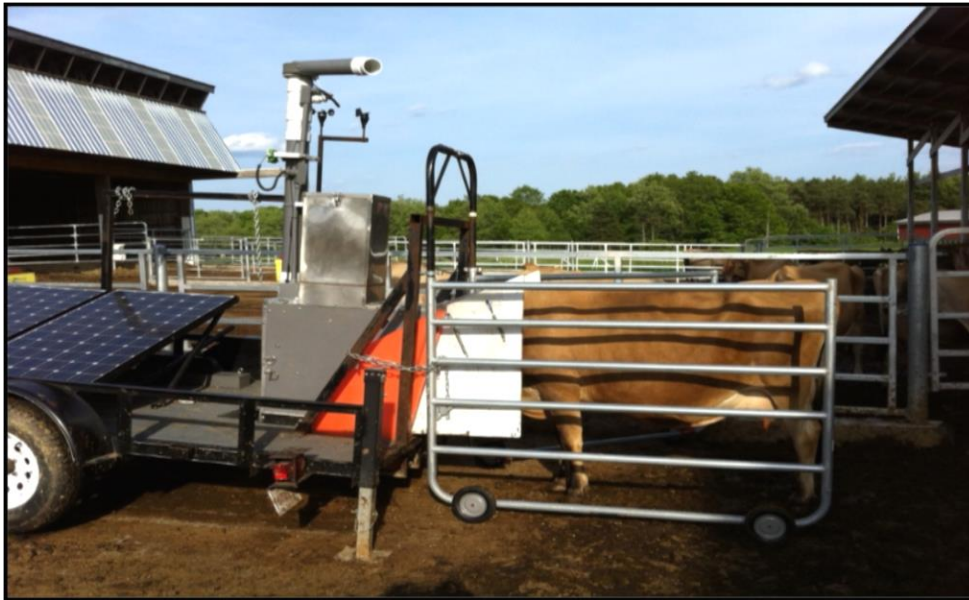
Figure 4. The GreenFeed solar-powered, automated gaseous measurement unit at the UNH Organic Dairy Research Farm (Lee, NH)
