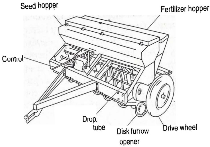
a. Grain drill for small grains that are sown in close rows
