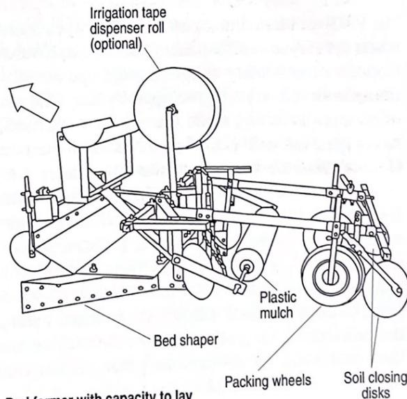
b. Bed former with capacity to lay drip irrigation and plastic mulch
