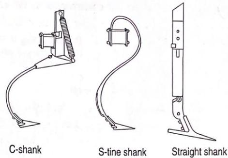
Shanks have a tool (such as a shovel or sweep) attached at the bottom. In general, C-shanks vibrate slightly; S-tine shanks vibrate vigorously; and straight shanks are rigid.
