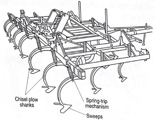
**Figure 9.2** Chisel plows
