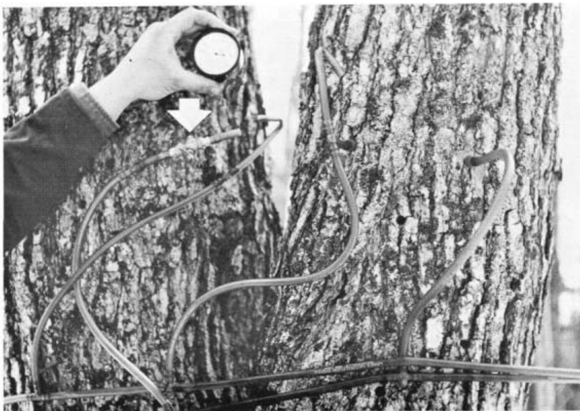
Figure 1b. Vacuum was measured in closed-tap installations after attaching gauge and opening petcock. (Arrow indicates petcock.)
