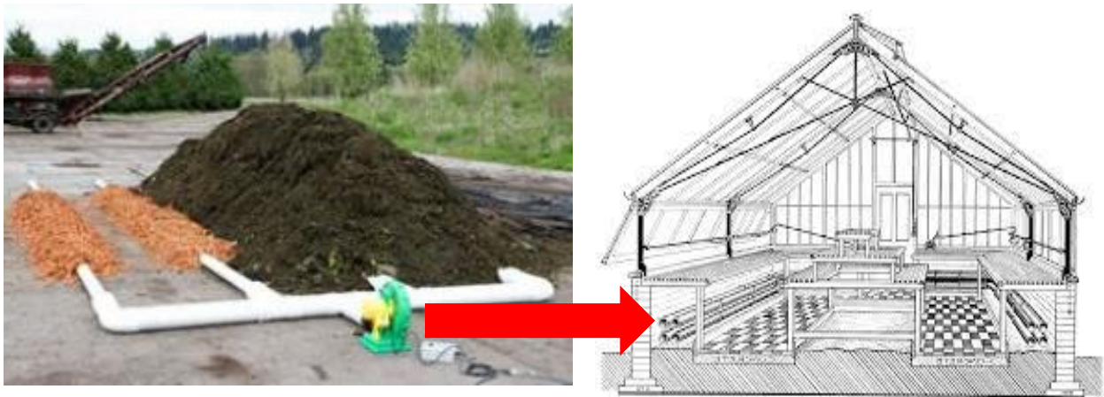
Figure E.3. Conceptual diagram of a high tunnel/greenhouse system heated by direct piping of vapor from an ASP system into heat transfer pipes within the structure.
