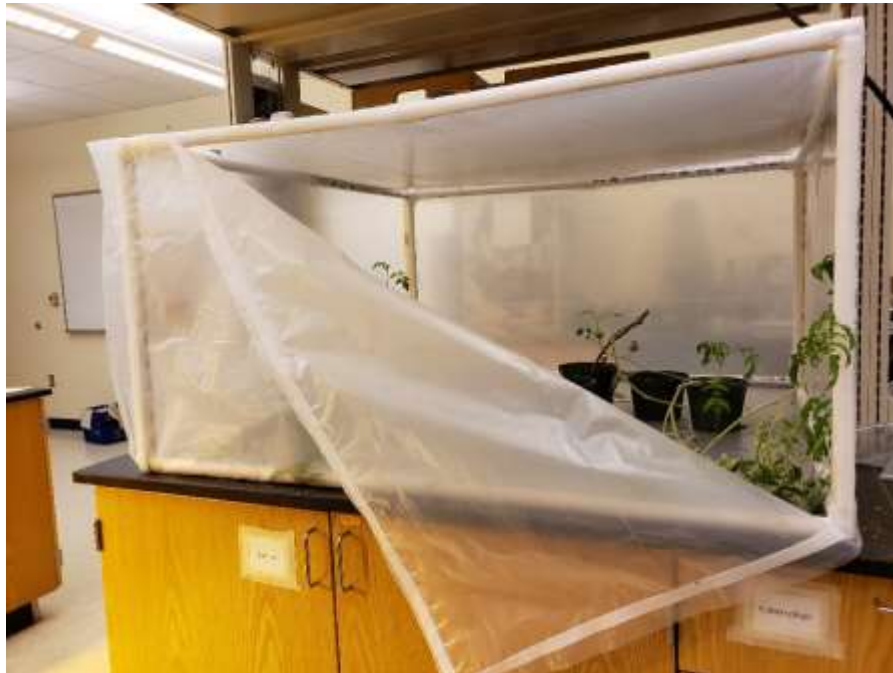
Fig. 2. Bench top humid chamber to keep tomato plants infected with PM and get new plants exposed to PM
