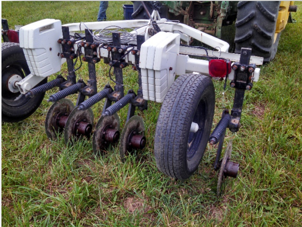
Veris 3100 used to map soil electrical conductivity
