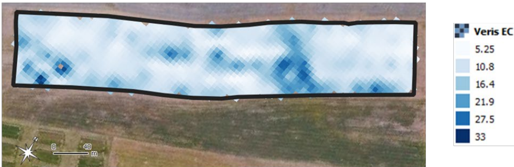
Figure 2. An interpolated surface of Veris EC readings measured before cover crop planting.
