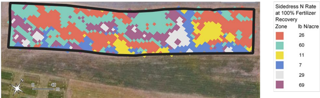
Figure 3. A variable rate prescription, accounting for differences in soil texture, soil organic matter, cover crop N content and cover crop C:N ratio.
