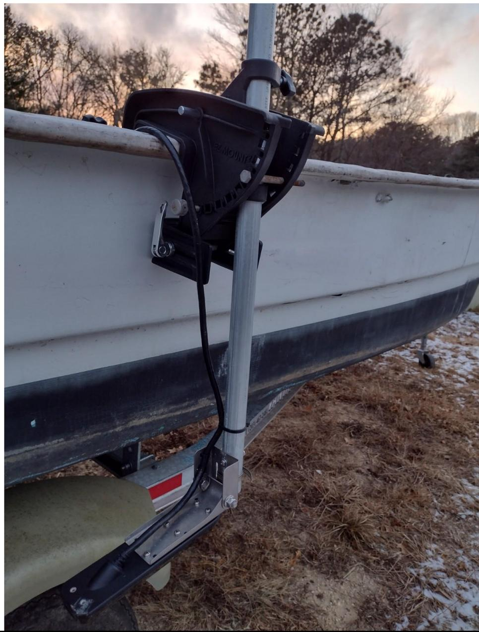
The fiberglass reinforced electric trolling motor mount with transducer mounted pole clamped to the bow of our 19' Carolina Skiff
