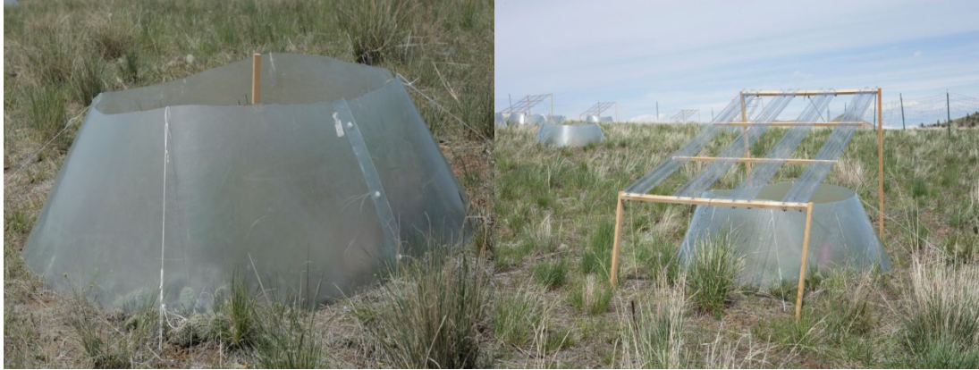
Figure 1-2. Photo of the “Hot” open top chambers (OTCs) (on left) and “Hot+Dry” OTCs and rain out shelters (ROSs) (on right) for Objective 1.
