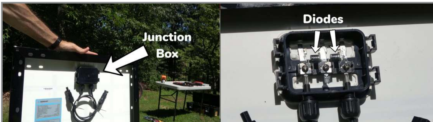
Figure 3. A junction box a) is visible on the back side of a solar module; and b) has been opened to allow access to the mounting terminals and internal bypass diodes.
