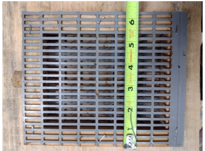
Image 2. Drone banking cage showing the width measurement.
