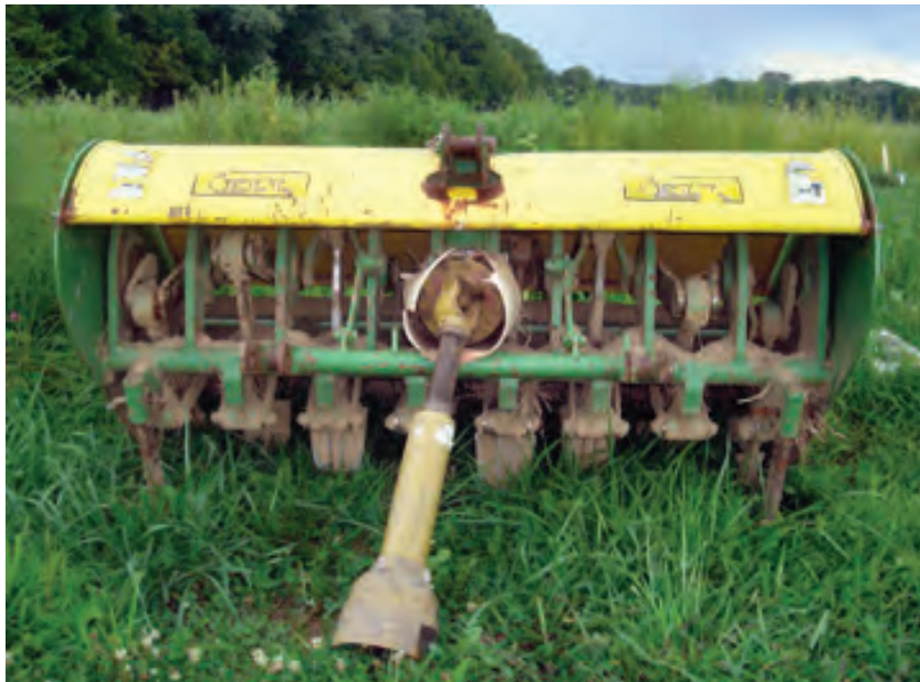
A Celli spading machine at Pennypack Farm and Education Center in Horsham, Pennsylvania. Photo: Andy Pressman, NCAT
