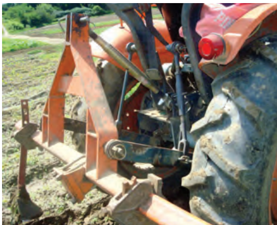
A three-point hitch with toolbar. Photo: Andy Pressman, NCAT
