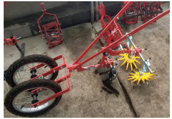
Terrateck wheel hoe with attachments. Photo: Andy Pressman, NCAT
