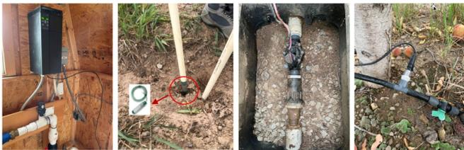
Figure 3. shows some of the components used in the system. From left to right: pump controller, soil moisture sensors, solenoid valve, and pressure sensor. Images: Long He, Penn State
