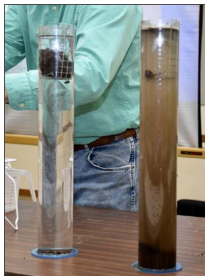
Photo: J. Johnson, Iowa NRCS This slake test shows that the soil on the right has poor aggregate stability, which could lead to reduced water infiltration and root penetration.
