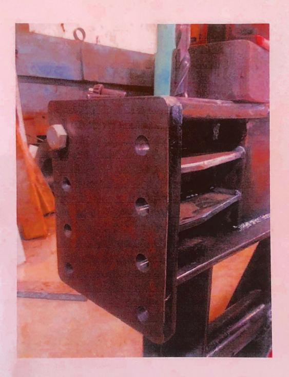
2. Welded 3/4 inch plate to the opposite end of the unit to use to bolt accessories to. Placed reinforcement gussets behind plated end on I-Beam to add additional support during operation of press under 30 tons of pressure. Fabricated an additional wedge attachment to be bolted to end plate with 3/4 inch bolts.
