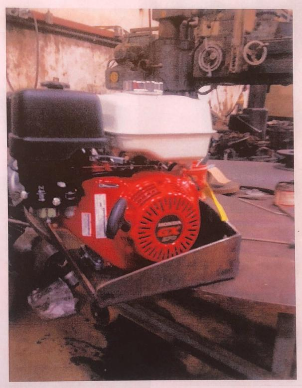
7. Engine placement- will be bolted to the mounting plate and attached to the hydraulic pump with lovejoy adaptor. (1/2"-1") Reservoir and Pump will be mounted on the other side of the plate.
