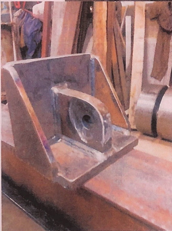
9. Proximal end of hydraulic cylinder mounting bracket and plate attachment for manure press box.
