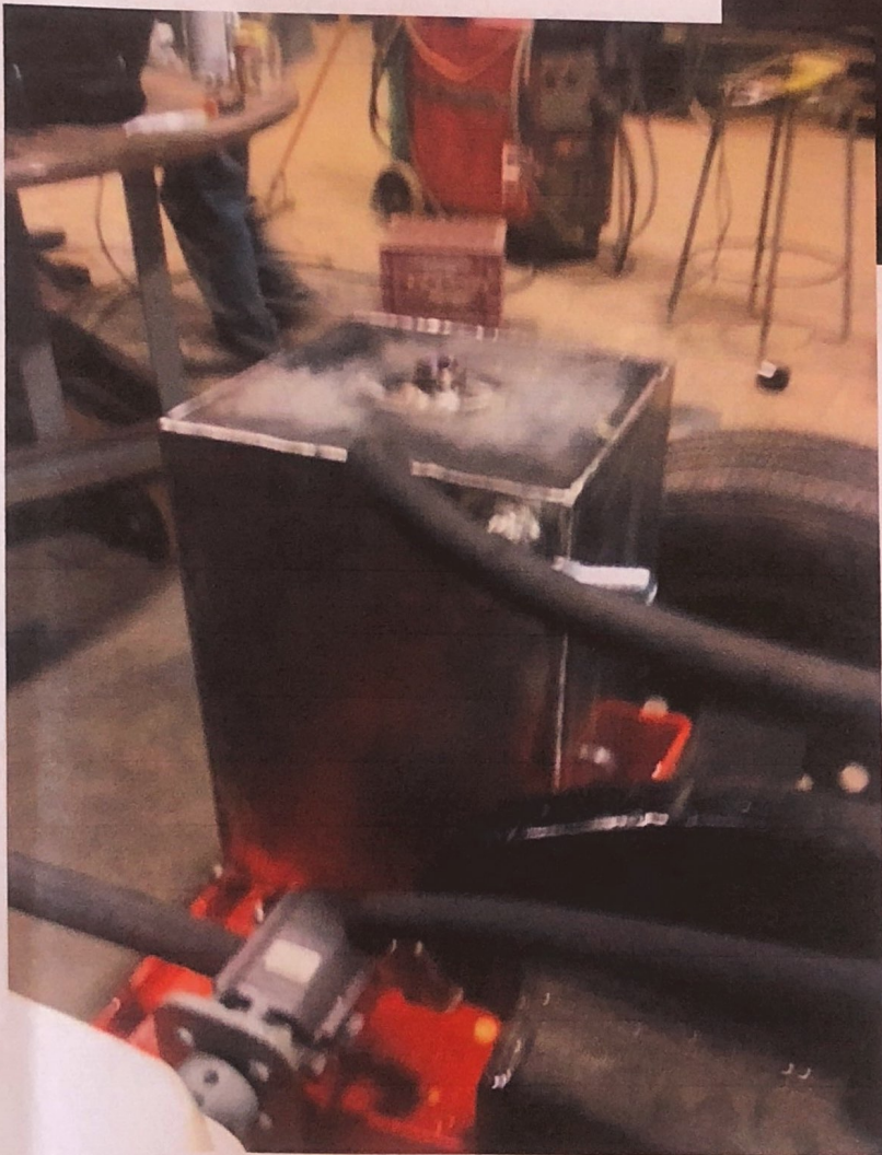
Hydraulic reservoir 5gallon capacity
