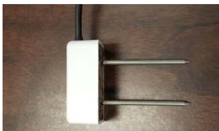
Fig. 3. Three examples of sensors that estimate volumetric water content: A) Spectrum Technologies TDR 300, B) Decagon Devices ECH20, and C) Decagon Devices GS1.
