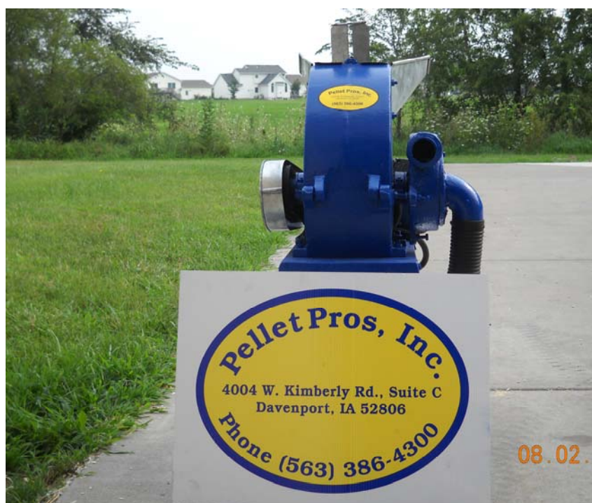
Small Scale Pellet Pros Hammermill. 130lb/hr capacity
