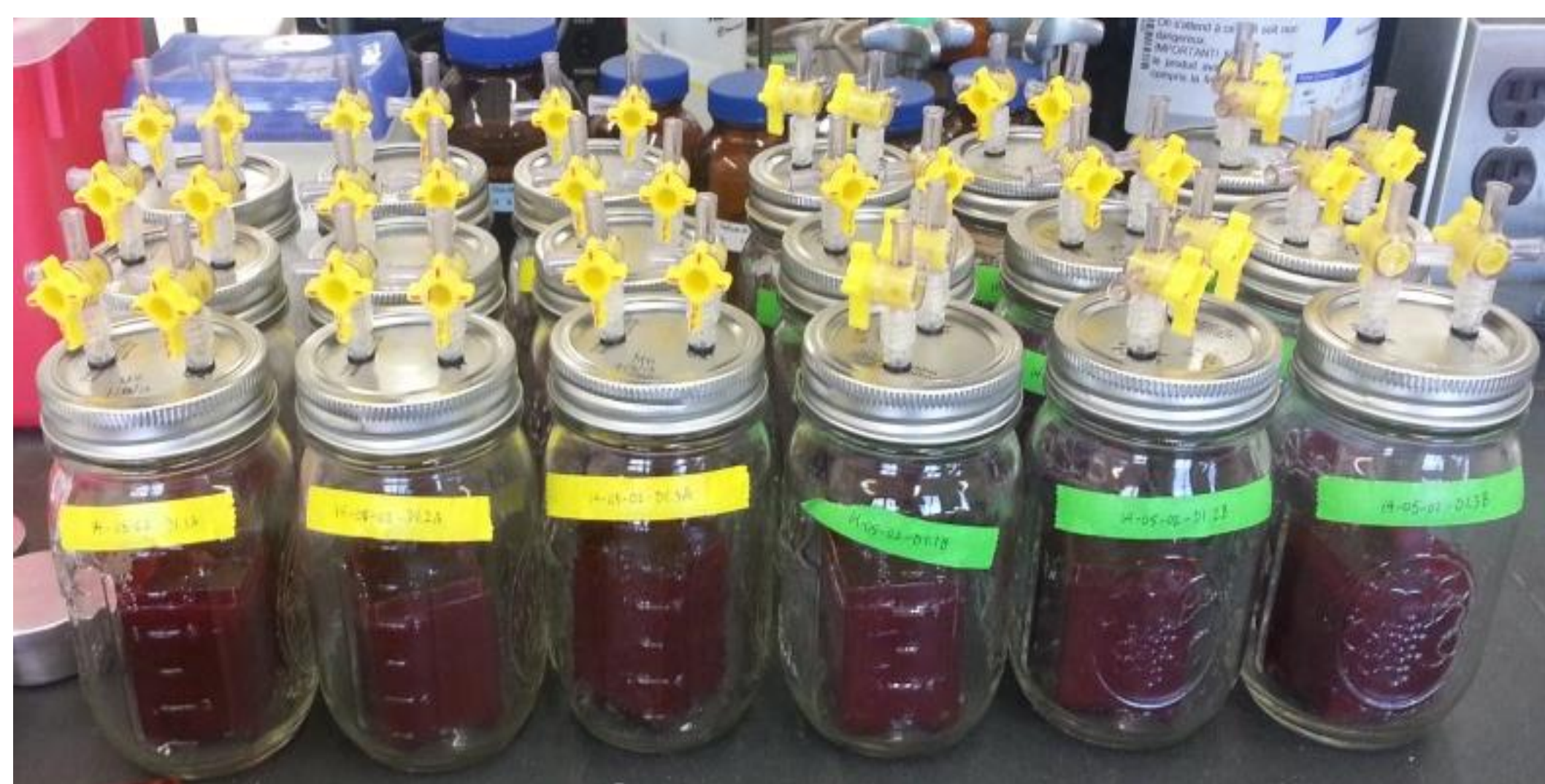
Figure 2. Soil incubation chambers equipped with headspace sampling ports.
