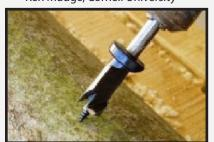
High speed drill bit for angle grinder. (Ken Mudge, Cornell Univesity)
