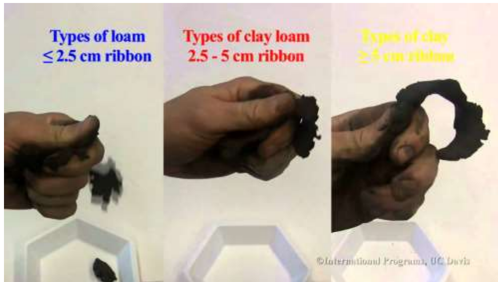
Fig. 4: Forming and ribbon and how to determine texture class from length of ribbon
