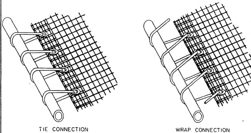
FIGURE 2. CABLE, PIPE, OR REBAR CONSTRUCTION
