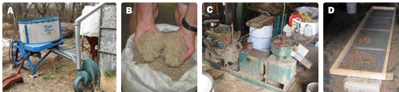
Figure 11. Equipment used for making pellets at Wood Crest Farm: (a) bale grinder and hammer mill, (b) ground switchgrass for pelleting, (c) pelletizer, (d) cooling rack.
