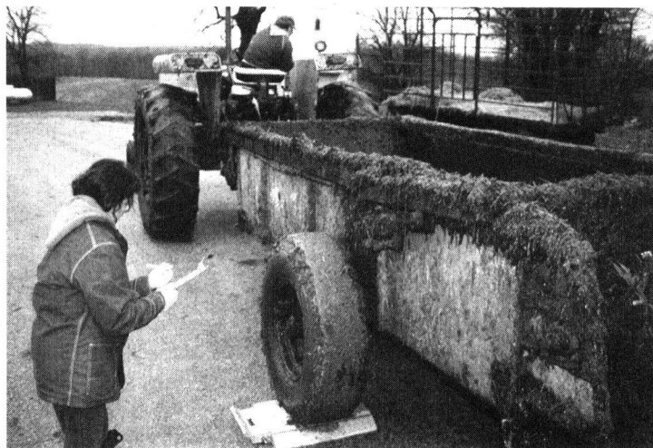
Karen Talarczyk, NPM SW regional specialist, records the weight of an empty manure spreader as part of a spreader calibration method.
