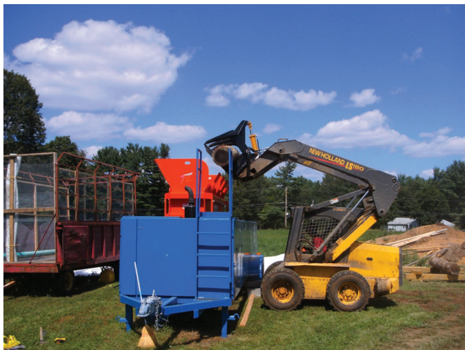
Figure 1. University of New Hampshire wood shaving machine being loaded. Color version available online.
