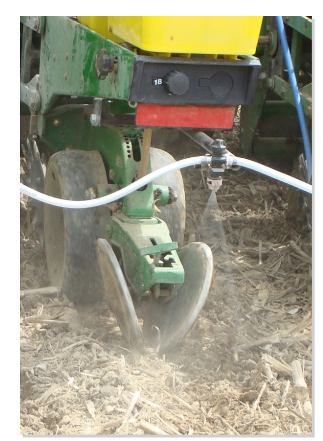
Herbicide being banded over row.
