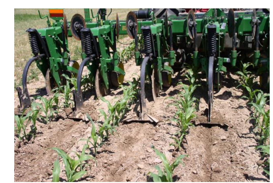
High-residue cultivation between crop rows.
