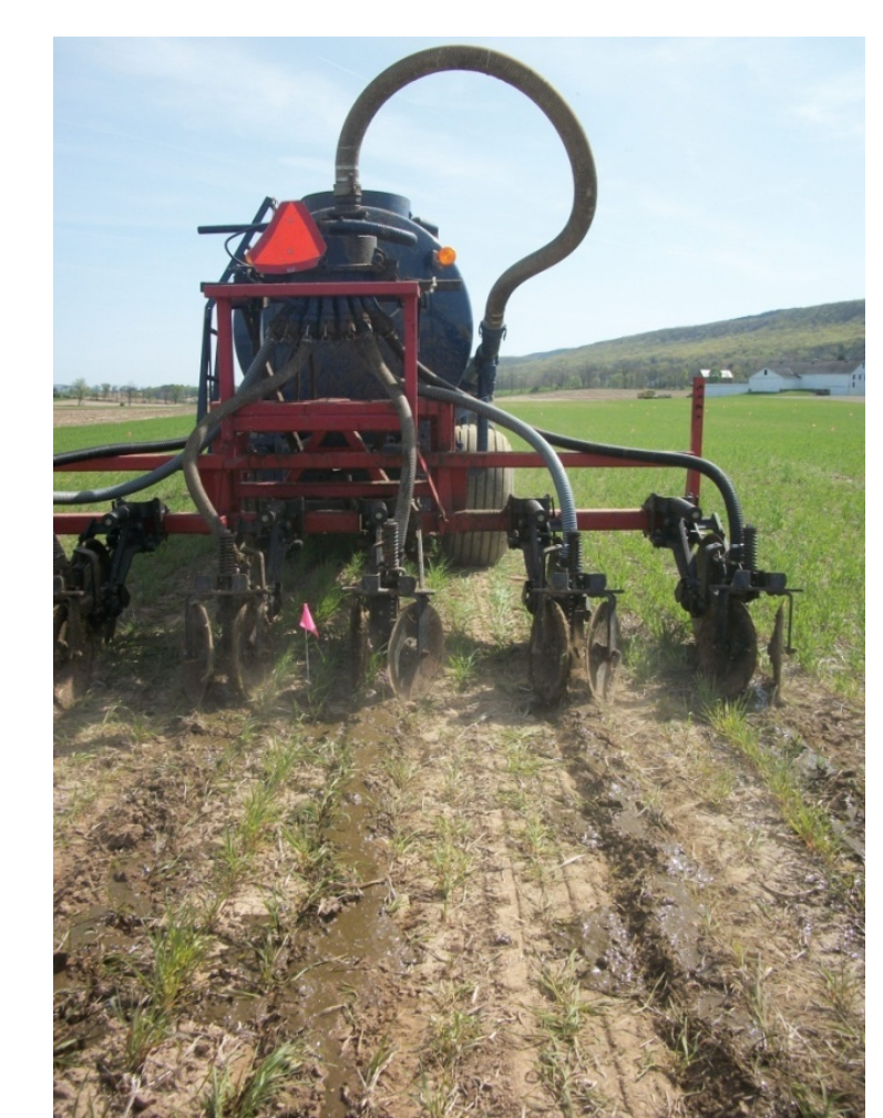
Shallow-disk manure injection.
