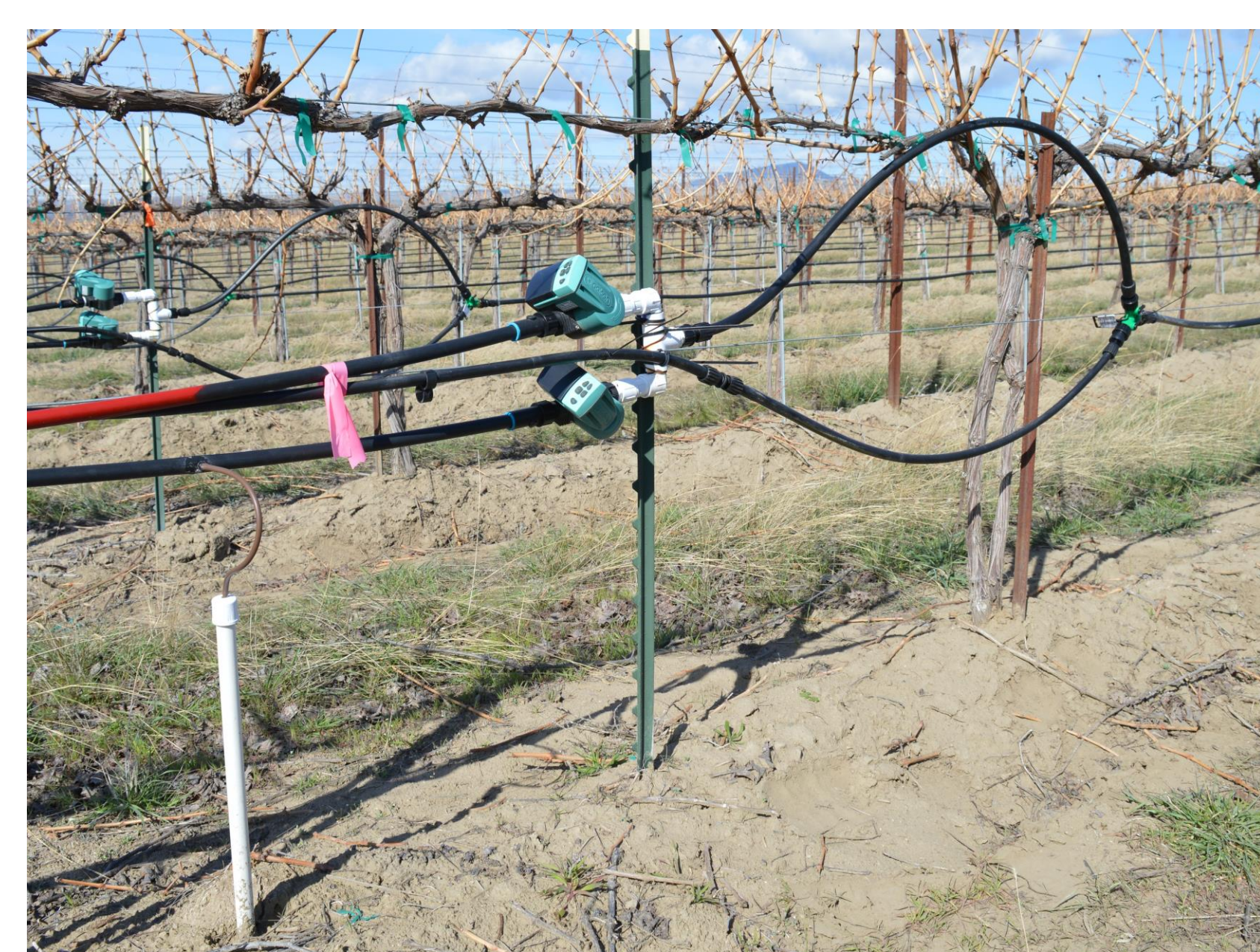
Figure 2. Battery powered controller in field site
