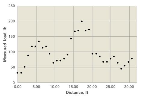
**Figure 1.** Contact force of depth wheels on soil during 30 ft of travel (about 4 sec at 5 mi/h or 3 sec at 7 mi/h.)
