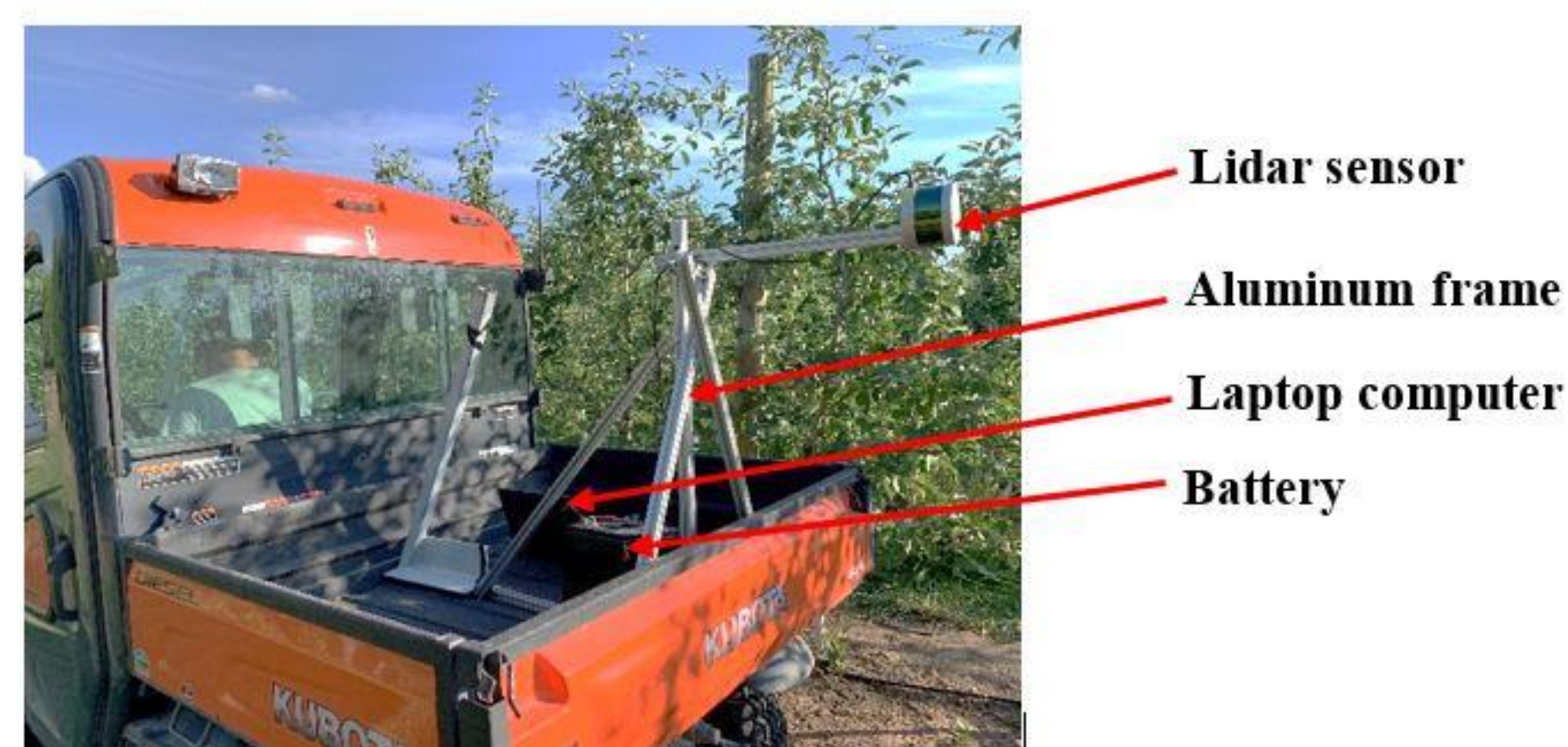
Fig 3. Scanning tree from both-sides using a LiDAR
