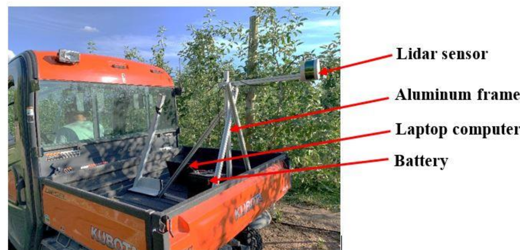
Fig 3. Scanning tree from both-sides using a LiDAR
