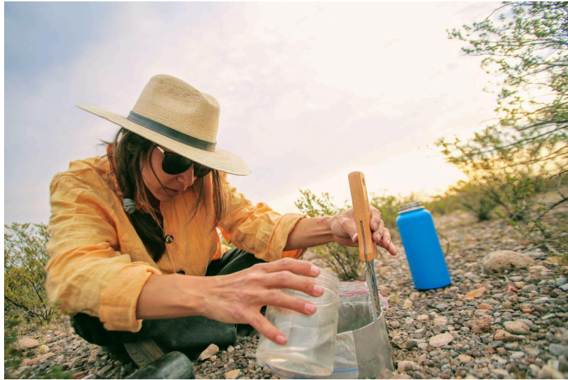
Figure 4: CRI Project Manager Garcia measures the infiltration rate of arid rocky soils.
