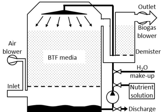
**Figure 1.** Cross-section of typical biogas biotrickling filter design. Raw-biogas enters at the inlet and treated-biogas leaves the outlet. Trickling phase (sulfur-laden nutrient water) is recirculated, and periodically discharged and replenished with make-up water and nutrients.
