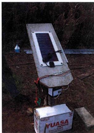
The fence is charge with a flexible solar panel.
