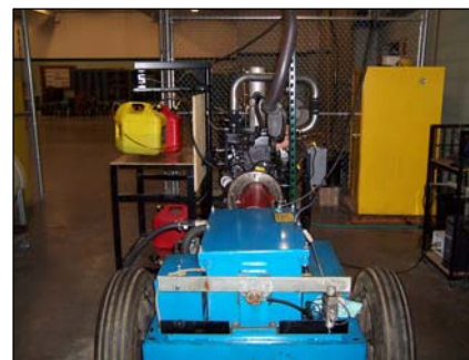
Figure 1. Major components of the diesel engine test stand and fuel stand, engine and dynamometer.
