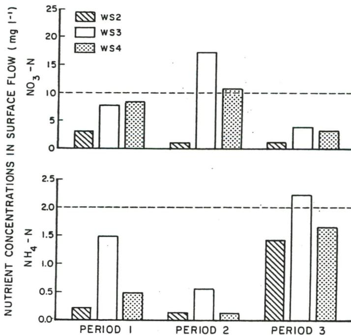
Figure 2. Runoff-weighted concentrations of  $\text{NO}_3^-$ -N and  $\text{NH}_4^+$ -N in surface flow by seasonal period. Dashed lines represent current water quality standards (from Alberts and Spomer, 1985).
