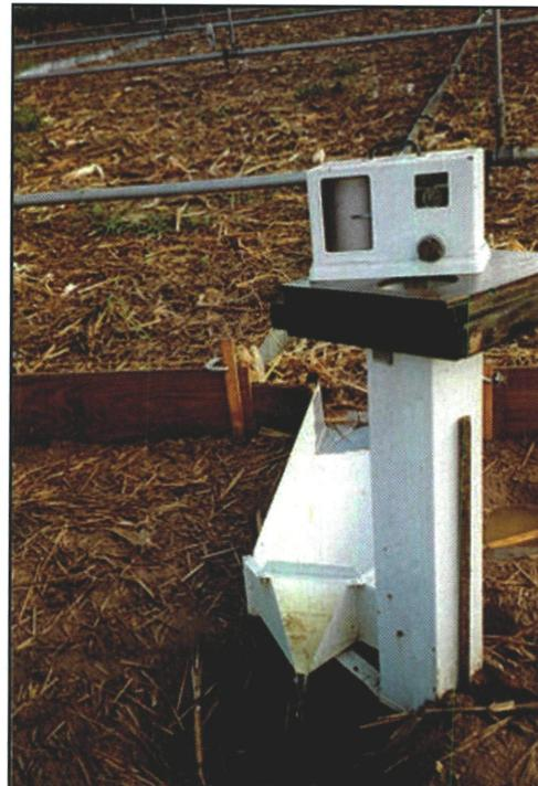
These flumes funnel excess stormwater from each research plot through a flow meter that measures the water's volume. Water samples from the flumes are used to evaluate the levels of sediment, nitrogen, and phosphorus washed from each plot.
