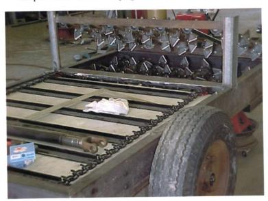
Next was the chopper. I wanted to keep as many of the parts for this machine as I could stock items. So the machine could be built with over the counter parts. For the chopper I decided to use common sickle bar knifes. These are available in many different styles and sizes. I ran one set of shafts flat and the other on an angle so that as the straw feeds farther into the machine it would chop the entire mat from the round bale.
