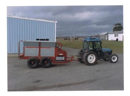
b. Straw Chopper – This is the part of the project that required the most work. I had to design and build this machine from scratch. I needed a machine that would handle a large round bale – unroll it – chop it – drop the chopped straw into the middle of the row.
