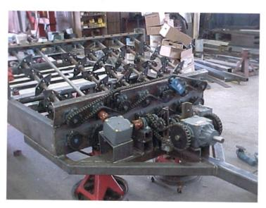
Now all that had to be done is frame everything in and run the hydraulics to operate the table chain. I also added a flow control to the hydraulic system so I could adjust the table chain speed (how fast the straw would feed into the chopper). This way I could match the speed that the straw would feed to the speed in which the tractor is traveling.
