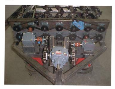
What I did here was to come from the tractor's PTO with a shaft turning at 540 rpms and go into a 1 to 2 gear box that splits it 2 ways. Then out of the gear box with a 26-tooth sprocket to a 13-tooth sprocket to again double the PTO speed. By weaving the chain over and under the sprockets for the chopper shafts it makes them work in opposite directions so the blades work against each other to chop the straw.
