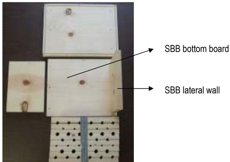
**Step 2** - Determine the location of the second lateral wall by placing the SBB nesting block in its position.
