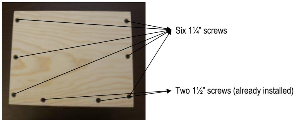
**Step 5** - Secure the back wall to the bottom board by using two 1½” screws.
