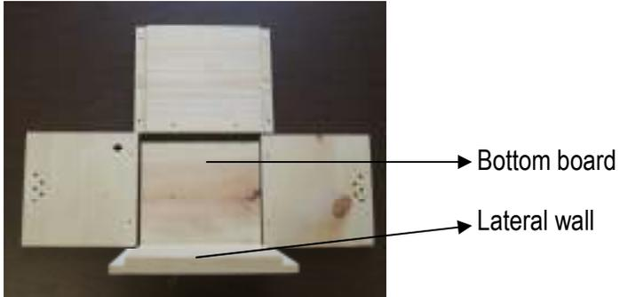
**Step 2** - Secure the second lateral wall to the bottom board by using two 1½" screws.
