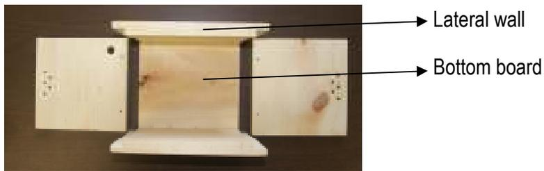
**Step 3** - Secure the front wall to the bottom board by using two 1½" screws.
