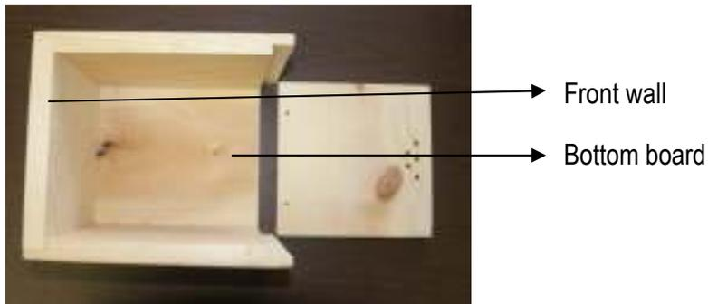
**Step 4** - Secure the lateral walls to the front wall by using six 1¼" screws.
