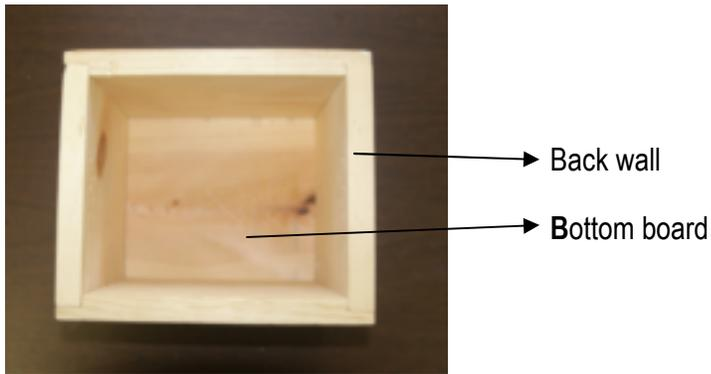
**Step 6** - Secure the lateral walls to the front wall by using six 1¼” screws.
