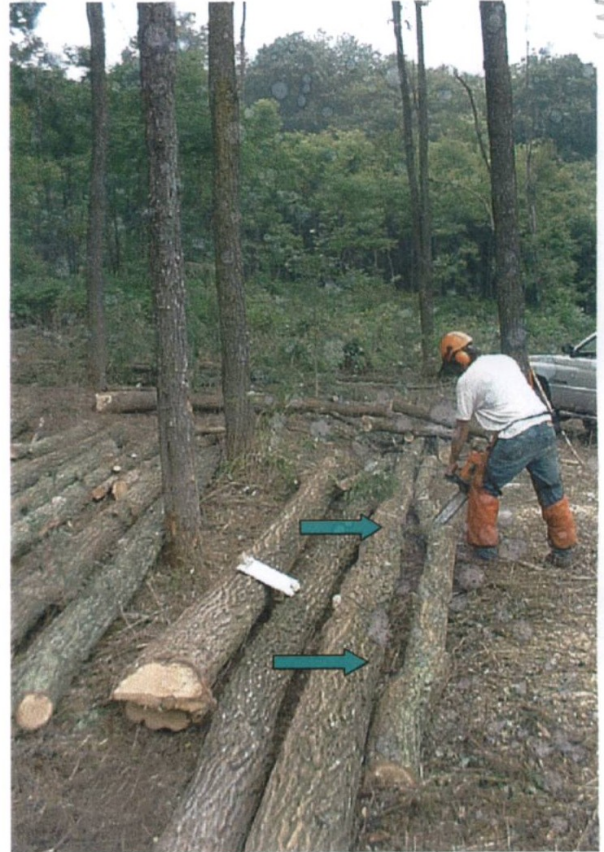
By cutting between crooks, useful short beams can be harvested from crooked, common locust logs
