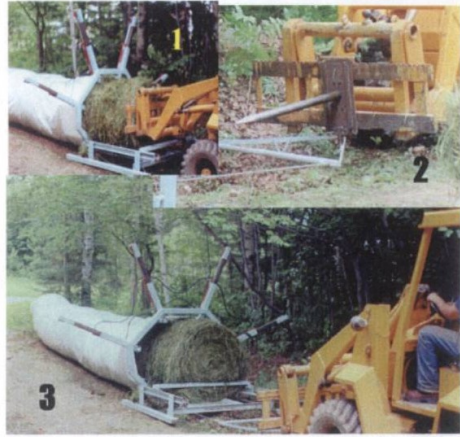
Fig 4. (1) Loading the bale onto the bale carriage. (2) Inserting tab into triangle. (3) Pulling triangle back, pushing bale into tube. Note the bar pushing on bale.
