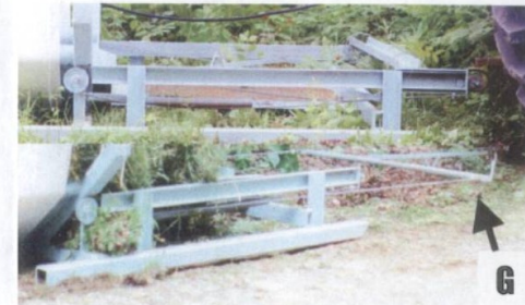
Fig 7. The second cable attached to the pusher bar (E in Fig 6) wraps around the rear pulley (B in Fig 5), continues forward, and connects to the pulling triangle (G).
