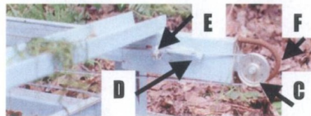
Fig 6. A steel cable runs from the front of the spring, around the front pulley (C), and attaches to the pusher bar (D). A second
