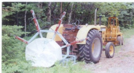
Fig 1. The hydraulics of a tractor are used to open the arms and stretch the bag.
