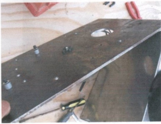
The four screws that hold the big pulley on, and the zirc fitting sticking through the center whole.
