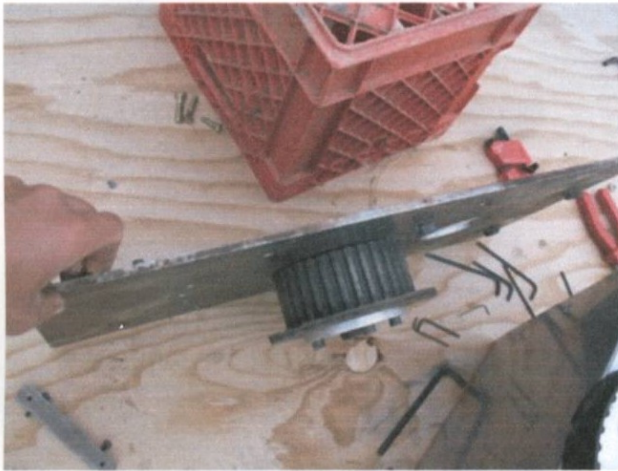
Big pulley screwed on to the center of the plate. Note it's screwed on to the side that has the nuts welded on to it, and the pulley is against the plate (with the zirc fitting sticking through the hole).
