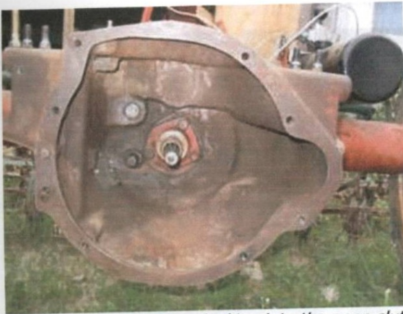
(Back View of the tractor, looking into the open clutch housing after unbolting the engine.)
