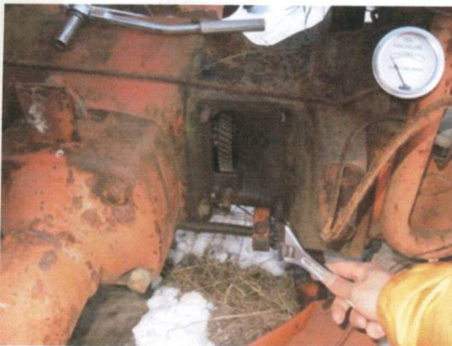
Unscrewing the clutch lever. The gear cog you see above ran the original hydraulic pump (more on that later.)
