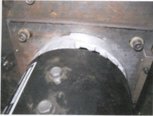
The four screws holding the motor on to the main plate. The holes are much larger than the screws so you can move the motor around.
