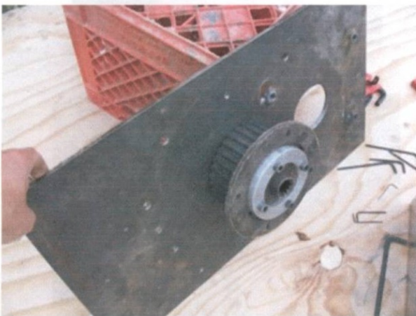
Another image of the big pulley screwed on to the center of the plate
