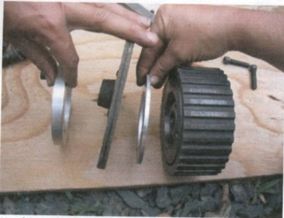
Attaching the pulley assembly to the clutch disk (we have an extra ring in this picture).
