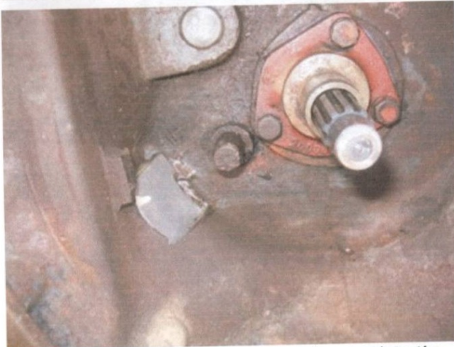
View from INSIDE the clutch housing. Look to the lower left to see the small aluminum scrap we used to patch the hole left over from removing the clutch lever.
