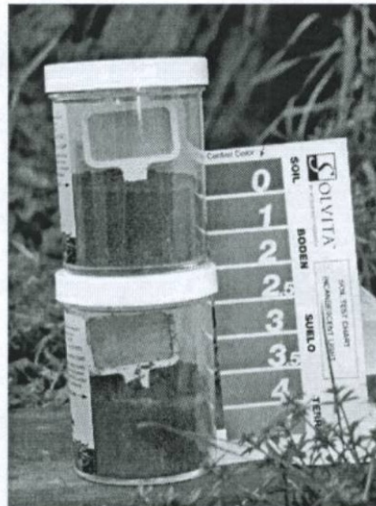
The Solvita soil life test used to measure soil microbial activity. Carbon dioxide production is graded according to color of the palates inserted into each jar.
