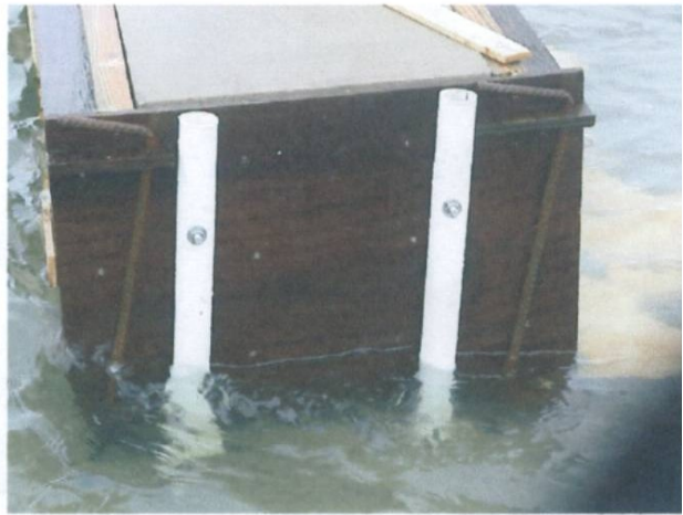
Figure 8. Modifications to secure upweller unit include these PVC pipes that were drilled through and attached directly to the upweller.
