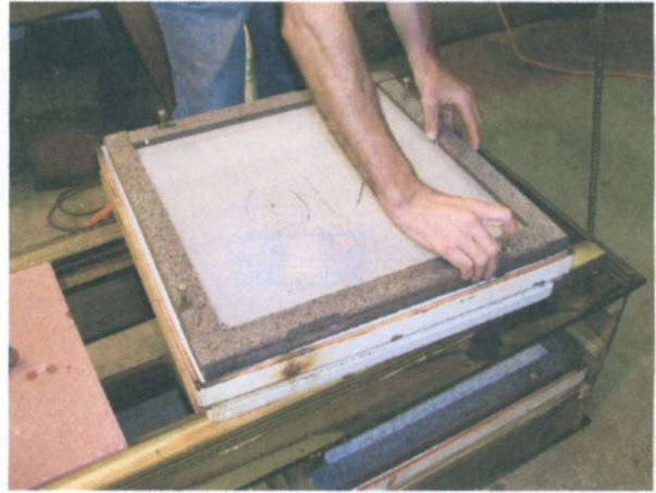
Figure 2. Close up of how upweller screen fits into upweller unit.
