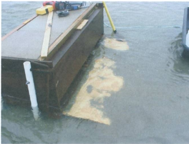
Figure 7. Modifications to secure upweller unit including wooden strapping on top of patio blocks and plywood anchor sheet attached to bottom of unit.
