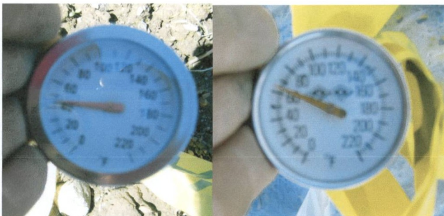
20 degree difference in soil temperature at 5" depth, May 4, 2007, 3 days before removal of plastic. Difference at 12" is 18 degrees.
