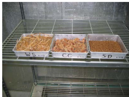
Figure 1 - Wheat straw, corn cob, and saw dust samples prepared for drying and moisture determination.
