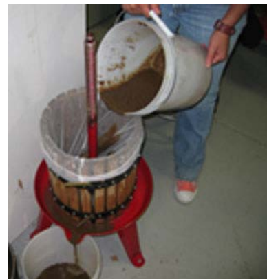
Figure 17 – Putting post-hydrolysis sample in filter press
