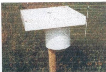
Figure 11. Fabricated solar radiation shield for air temperature/relative humidity data logger in weather station.
