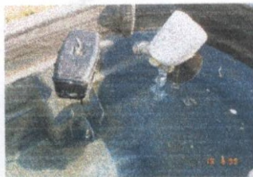
Figure 14. Full flow water level control device on left and float assembly for trough water temperature data logger on right.
