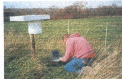
Figure 19. Digital data generated by field instruments was retrieved and transferred via a laptop PC to the office for storage, reduction, and later analysis.
