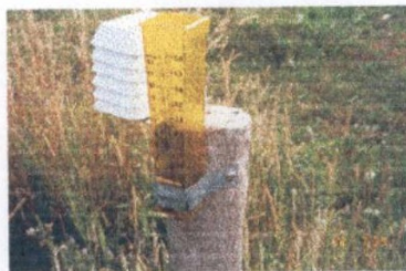
Figure 12. Rain gauge and sun shield for backup air temperature data logger.
