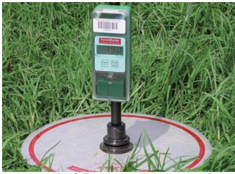
Figure 3. The falling/raising plate meter for estimating available forage in a pasture.
