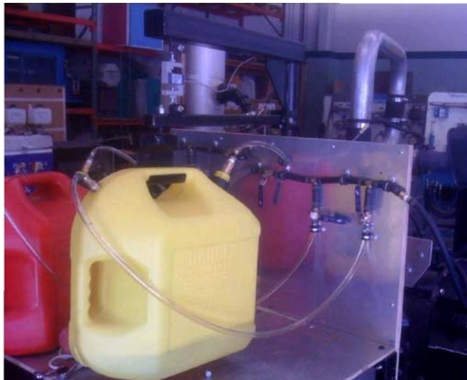
Figure 3. Fuel stand that shows the fuel lines to the experimental fuel and base fuel containers and an online weight measuring unit using a load cell connected to the data acquisition system.
